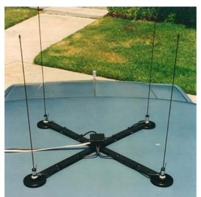
The problem was not detectable with an ohmmeter, but I could observe differences in pulse waveforms on the whips with an oscilloscope. That antenna version has chrome plated hex upper nuts and black whip-holding caps with hex-head setscrews. If you have one, I recommend that you add tape or other insulation at the crimp ends of the lugs at the whip bases to avoid shorts.
